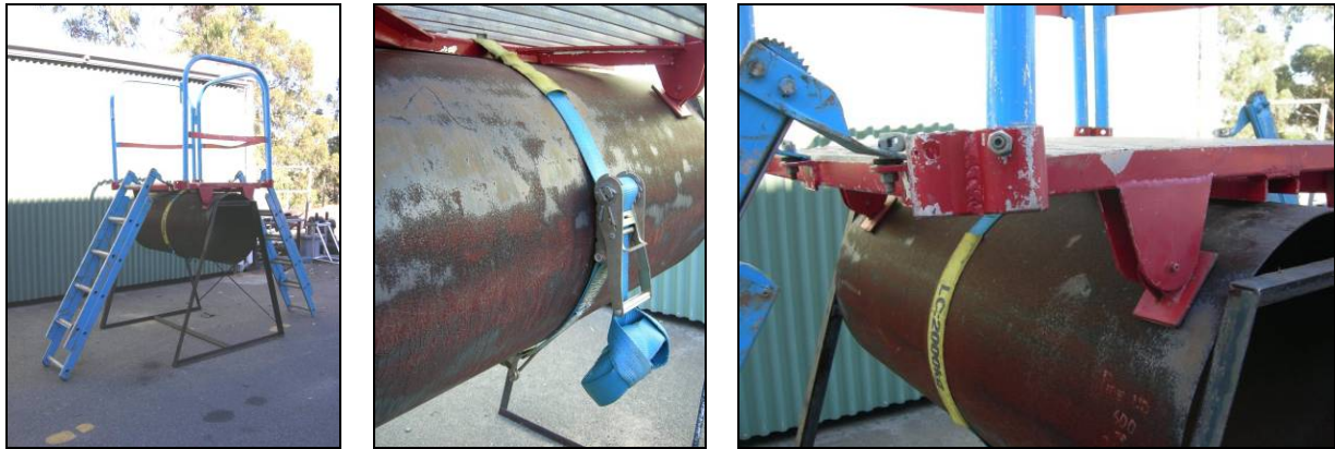
Example of a Portable Pipe Access Platform (Available from Central Workshops)
