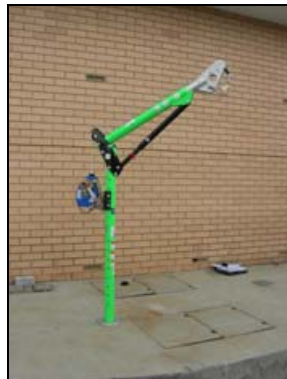
Portable Davit in Flush Mounted Base
