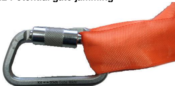
Fig 3.2 Potential gate jamming
