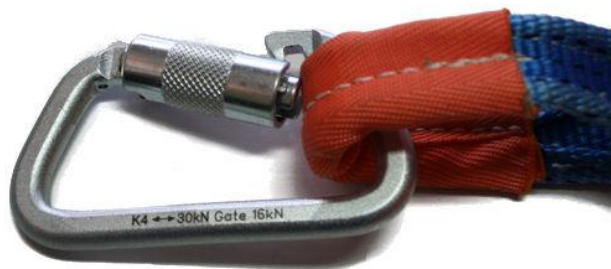
Fig 3.1 Potential gate jamming
